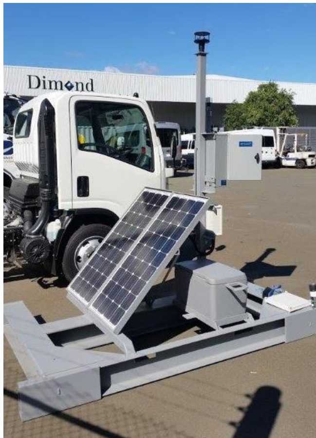
Figure 16: PM 10 monitoring instrument, batteries and solar panels installed on a mobile steel pellet.
