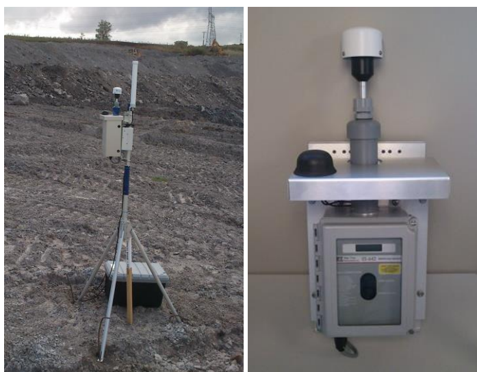
Figure 2 Typical nephelometer installations. The unit on the left is battery powered, while the unit on the right provides a close up of the instrument.
