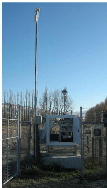
Figure 3 An example of a temperature controlled BAM enclosure with the doors open to illustrate the BAM inside
