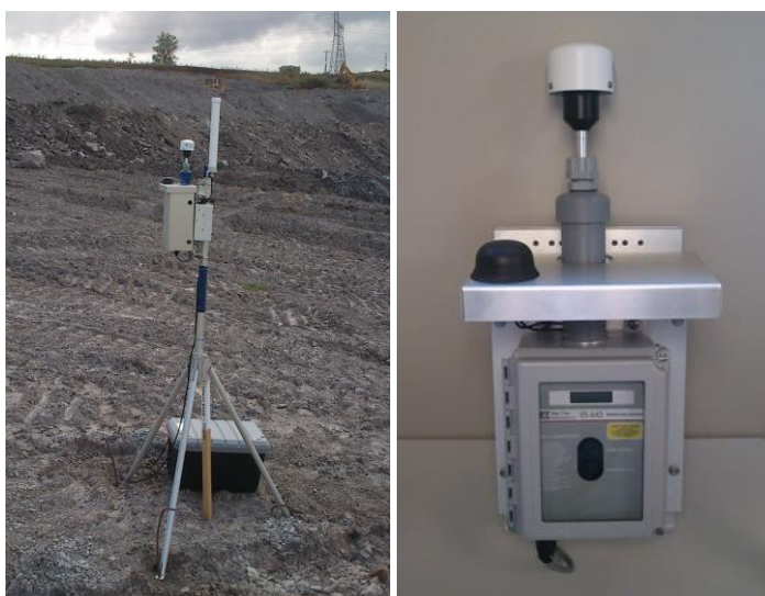
Figure 2 Typical nephelometer installations. The unit on the left is mains powered, while the unit in the centre is battery powered. The unit on the right provides a close up.
