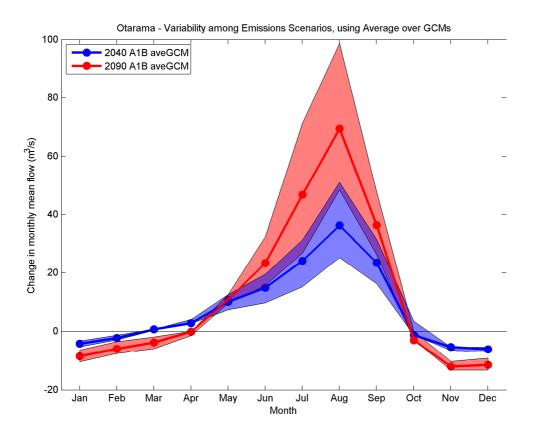
**Figure 3-1: Effect of emissions scenario on changes in monthly mean flow at Otarama.** Blue and red shading indicates the full range of results for 2040s and 2090s, respectively. Solid lines are for A1B emissions, which is the same case as used in Zammit and Woods (2011).<sup>1</sup>
