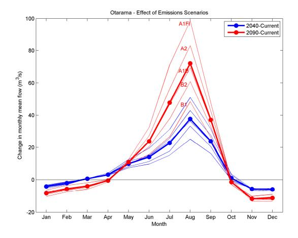
**Figure B1: Effect of emissions scenario on changes in monthly mean flow at Otarama**. The thin blue and red lines indicate the results for 2040s and 2090s, respectively. The thick lines are for A1B emissions used in Zammit and Woods (2011). The labels indicate the name of the emissions scenario for each model run in the 2090s<sup>2</sup>.
