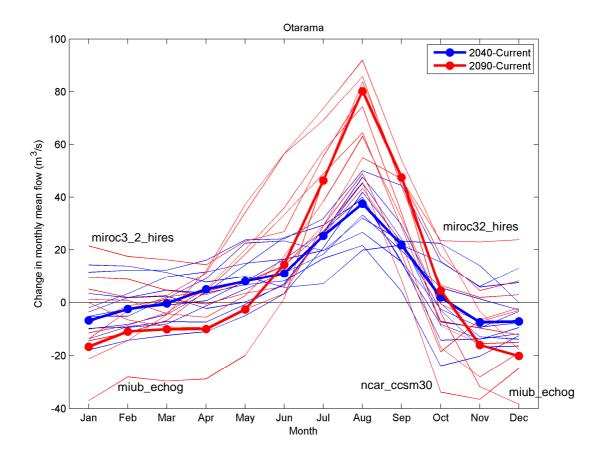
**Figure B2: Effect of GCM on changes in monthly mean flow at Otarama**. The thin blue and red indicate the results from each GCM for the 2040s and 2090s, respectively. Solid lines are for the average GCM climate used in Zammit and Woods (2011). The names of selected GCMs are attached to the traces for the 2090s
