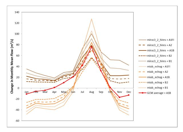
**Figure 3-3:** Effect of emissions scenario on flow in 2090s at Otarama, for two selected GCMs. Dark brown lines are for the miroc3\_2\_hires GCM, with various emissions scenarios (miroc3\_2\_hires was chosen because it produces the largest increase in mean flow). Orange lines are for the miub\_echo\_g GCM, with various emissions scenarios (miub\_echo\_g was chosen because it produces the lowest increase in mean flow). The red line for GCM average with A1B emissions is shown for reference.
