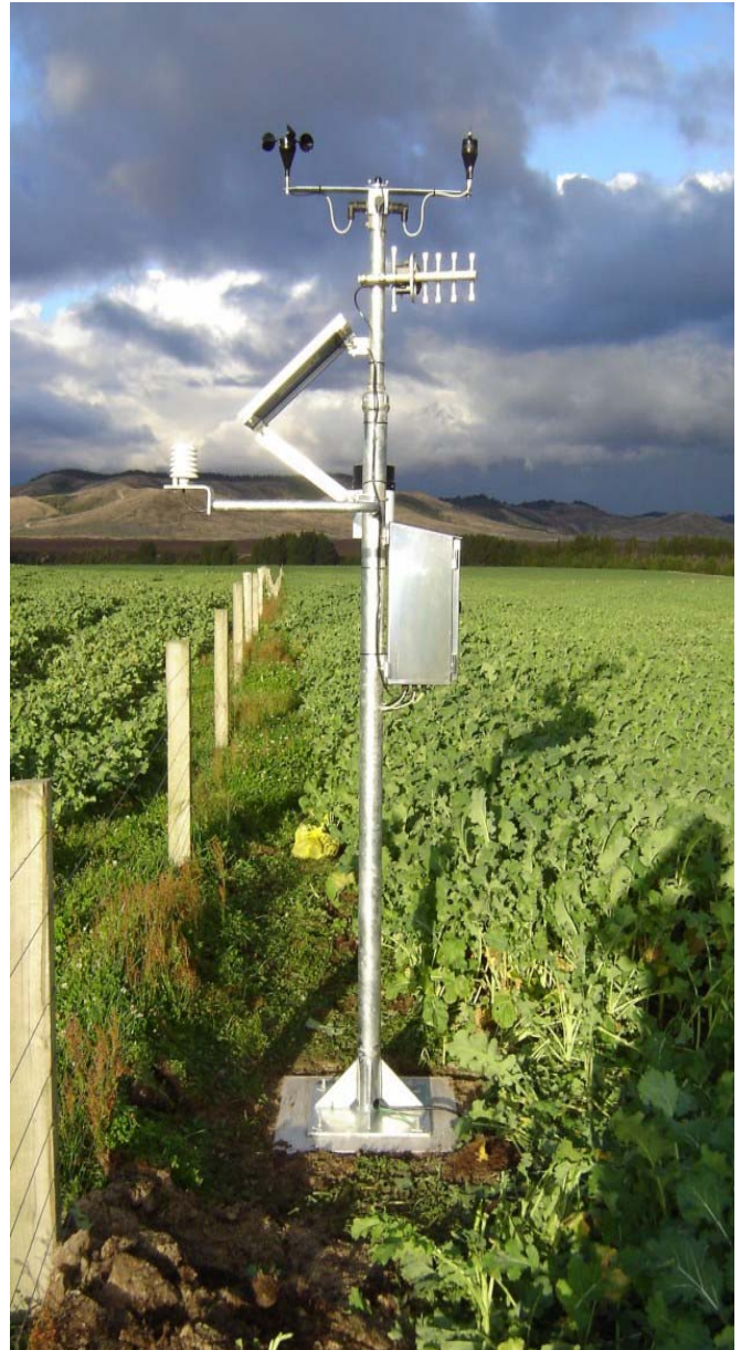
Ag/hort climate station measuring wind speed & direction, air temperature, humidity, solar radiation, soil moisture, rainfall, ET o and GDD
