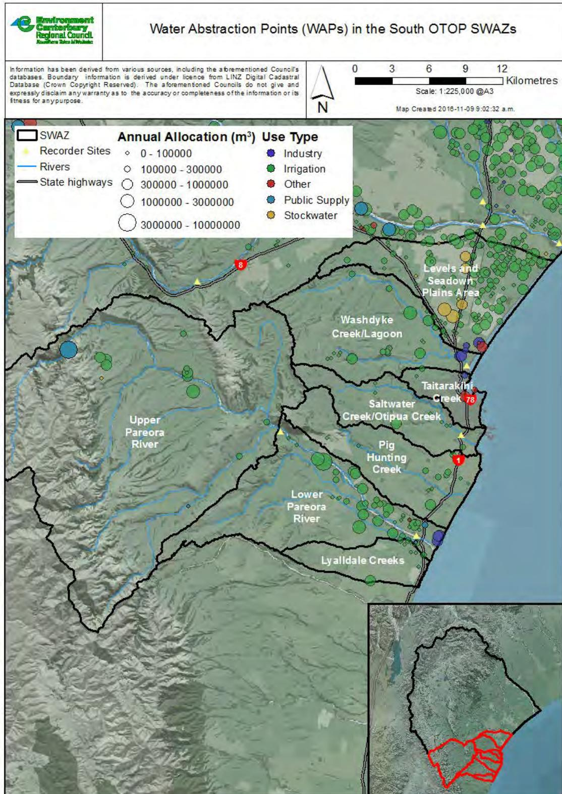
Figure 4-2: The Pareora SWAZ with all surface water and groundwater abstraction points with the symbol size representing the abstraction volume and the surface water recorders/minimum flow sites
